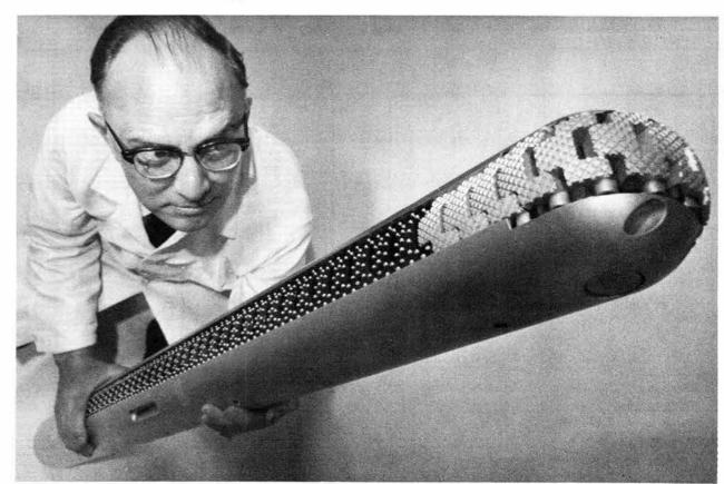
MODEL of experimental continuous chain bit, here held by Dick Ashmore (2325), shows cutting surface located on face of the chain, which is advanced to bring a new cutting surface into position. As the bit is rotated in the drill hole, the cutting surface scrapes the bottom and sides of the hole, gradually deepening it.
